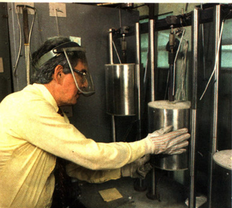
Robert A. Laudise removes furnace from a small hydrothermal autoclave prior to quenching the autoclave
